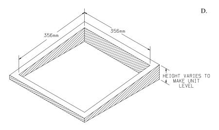
Once the heat pump has been leveled, some additional shimming may be required above the interior ceiling assembly. The heat pump and the interior ceiling assembly must have a squared installation relationship before they are secured together.
