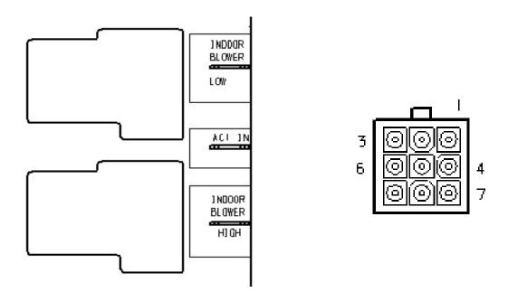
Note: Both High and Low Indoor Blower speeds operate on Circuit #1
