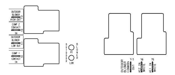
Note: These two sections of the p.c. board control both 115 volt (HOT and NEUTRAL) power legs to the OUTDOOR BLOWER.
