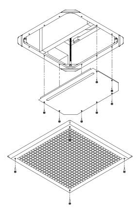
3. Install the supplied insulated duct locator plate as shown. Make certain the fiber divider board is fitted into the channel on the topside of the duct locator plate. Secure the duct locator plate with four of the retained screws.
