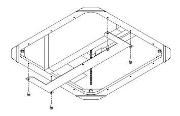
4. Remove the air filter assembly from the plastic interior Chillgrille<sup>TM</sup> by rotating the black fastener one-quarter turn. Attach the Chillgrille<sup>TM</sup> to the frame assembly with the supplied three sheet metal screws as shown. Tighten the three screws individually to affect a flush fit between the plastic grille and ceiling.
