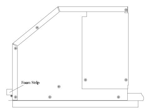
2) Install foam strip on the front of the evaporator housing just above the screw heads as shown above
