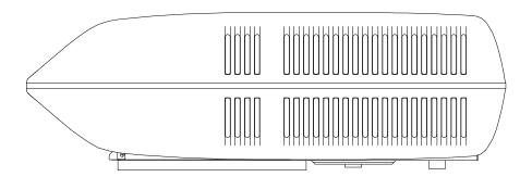
3) When installing shroud, work front lip over foam strip. Next pull shroud toward rear of unit and slide down over metal framework.
